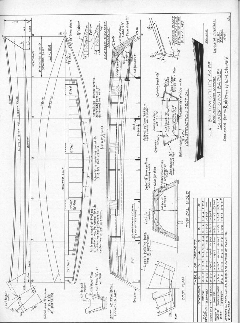
with one plank will certainly come out all right, and the width of plank needed can be made up out of two or three narrow planks. Join them with edge glued splined joints, or shiplapped joints, glued and copper riveted. Waterproof glue such as Cascophen must be used in both cases, of course, mixed and applied strictly in accordance with the maker's instructions.
