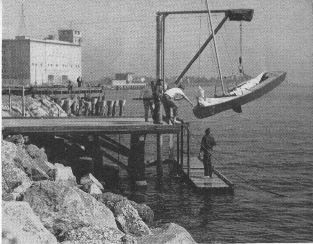
Newest and most prized acquisition of the growing Cabrillo Beach Yacht Club is the haulout crane. It is just big enough to handle boats up to and including Star class sloops
