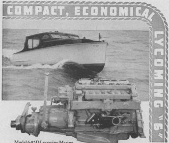
Model 6-85D Lycoming Marine Engine with reduction gear. Develops 85 Horse Power.
