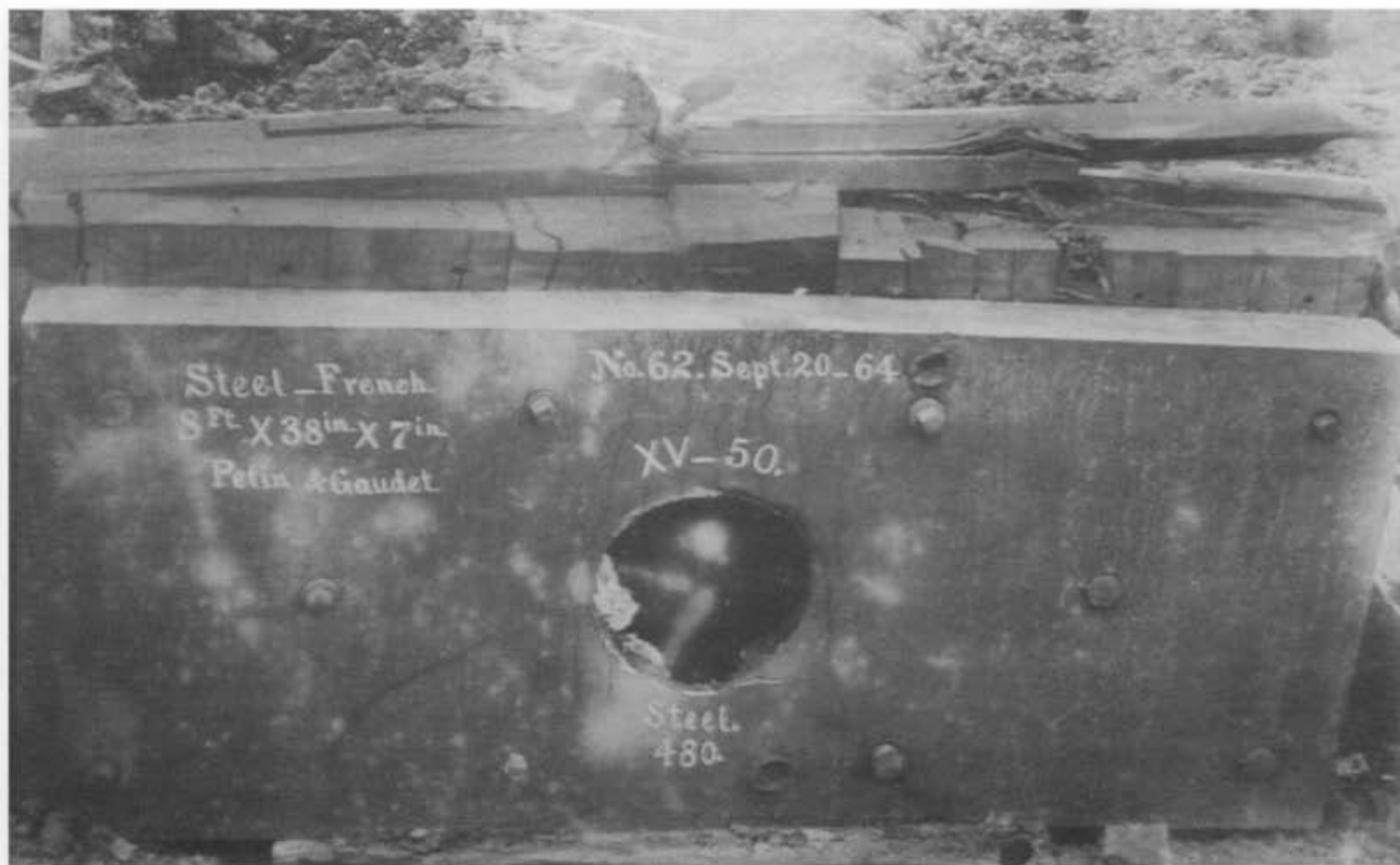
French 7-inch-steel armor plate target penetrated by a 15-inch shot. Courtesy of U.S. Archive Record Group 74, Entry 99 ("Reports of Target practice, 1862-1866"), vol. 3.
