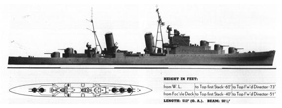
Figure 15 HMS Dido Antiaircraft Cruiser
