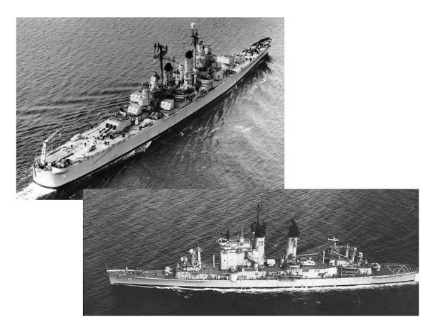
Figure 18 USS Columbus as CA 74 (top) and After Conversion to CG 12.
