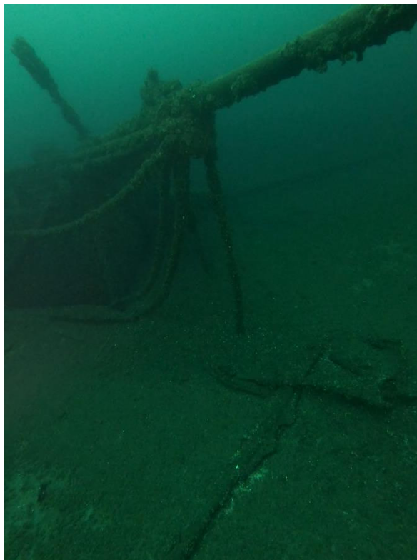
Figure 15. The bowsprit and jib boom of Katie Eccles with the bobstays, starboard and port bowsprit guys, jumbo jib stay and jumbo jib boom. Note the spreader and martingale spar.
