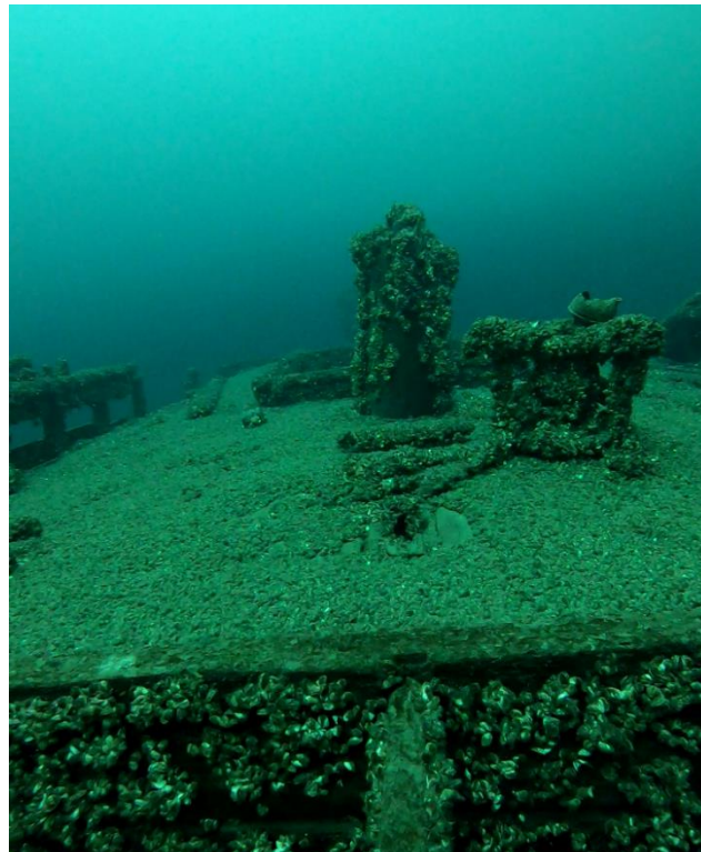
Figure 12. The centerboard pennant chock, pennant cable and centerboard winch with the mainmast looking aft
