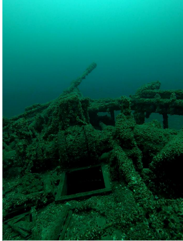
Fig.13 The foredeck with the pawl post, windlass and forecabin hatch
